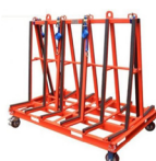
Transportable racks, bar-rows, trolleys and stillages: 5° - 6°
